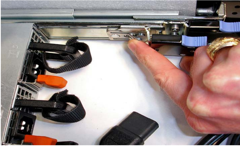
Figure 11: Replacing the Outer Power Supply
