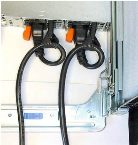
Figure 3: Routing Power Cables Through the Strain Reliefs
